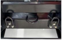
**Lifiting points and towing hook** Once the skip is in the raised position, you can use the 4 lifting hooks to lift the machine. A towing hook is also avalaible at the back of the chassis.
