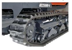
The KC250-4 track mechanism features tripple flange rollers. 8 track rollers are mounted on bogey type technology, it ensures great stability on slopes and rough terrain. The short pitch track offers smooth drive for an optimal comfort at high speed.
