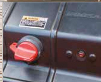
Battery cut-off switch
